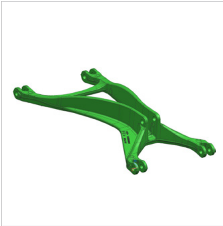
Refining of the optimized geometry in solidThinking Inspire
