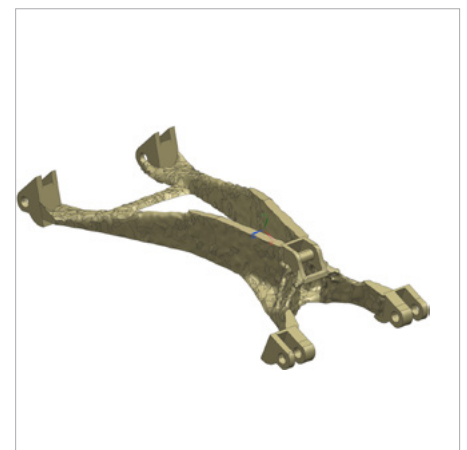
Based on previously defined loads and boundaries solidThinking Inspire calculates the optimal structure.
