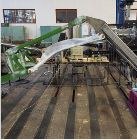
Physical tests of the casting part showed durability increased by a factor of 2.5.
