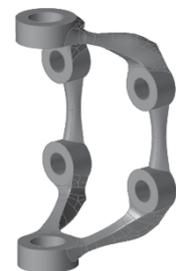
Figure 8: smoothed TO part generated utilizing PolyNURBS.
