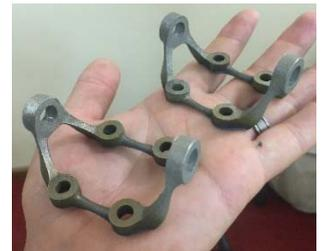
Figure 12: (l) standard test specimens and (r) initial pair of printed Ti64 C-Brackets.
