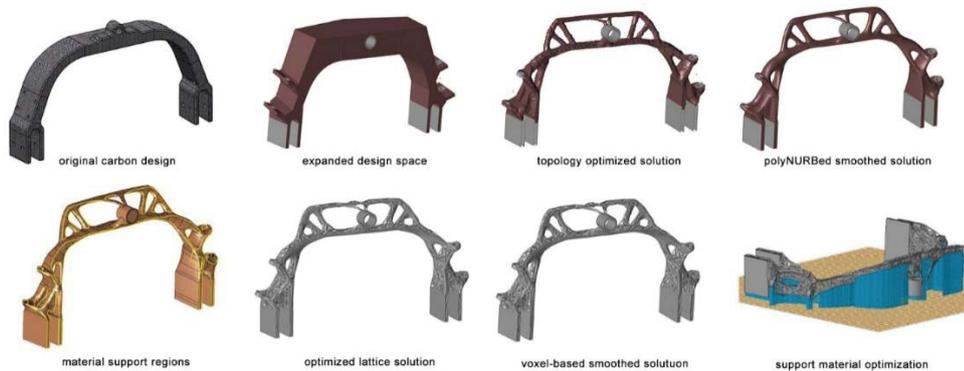
Figure 22: design evolution of Steering Arch from carbon to optimized & latticed Ti-6-4 AM design for face-down print.
