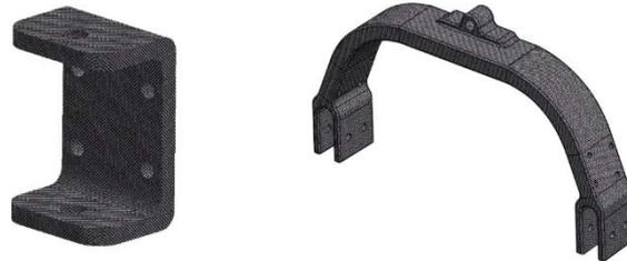
Figure 2: original C-Bracket & Steering Arch designs.
