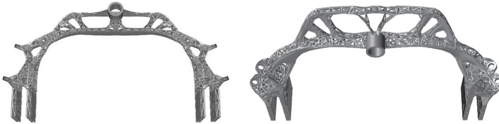
Figure 21: Smoothed Topology Optimized and Latticed steering arch, including solid 'shell' sections for support material connection (l) for upright orientation, and (b) for face-down orientation.
