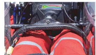
Figure 14: Original Steering Arch
