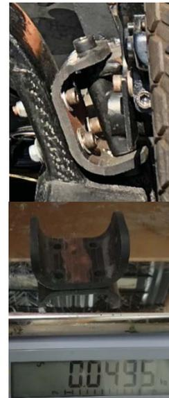
Figure 5: (top) C-Bracket in Eco-Car, and (bottom) mass of the original structure.
