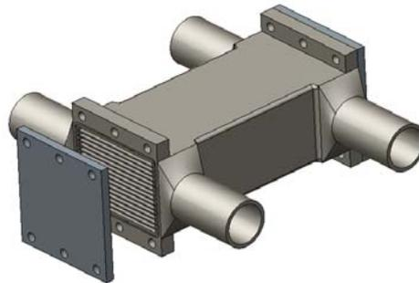
Figure 19: 3-D model with flanges.
