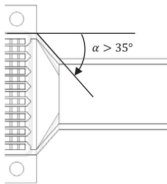
Figure 18: Transitioning section with  $\alpha$  larger than 35°.
