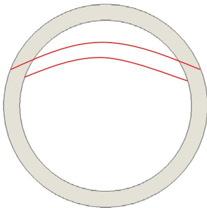
Figure 14: Circular section manufactured in a horizontal position without support.
