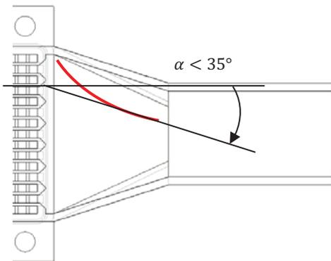
Figure 17: Transitioning section with  $\alpha$  smaller than 35°.
