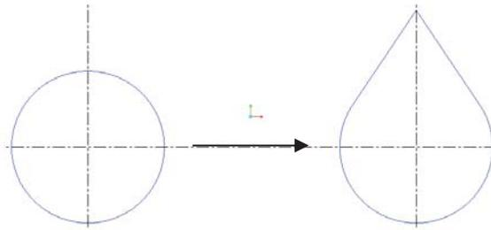
Figure 16: Shape adapted to create hole without supports.
