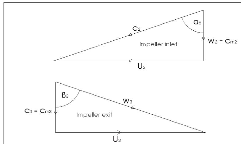
Figure 4 - Velocity triangles of turbine (adapted from [15]).
