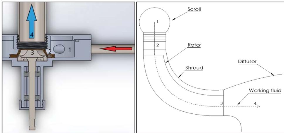
Figure 2 - Radial inflow turbine diagram (adapted from [15]).
