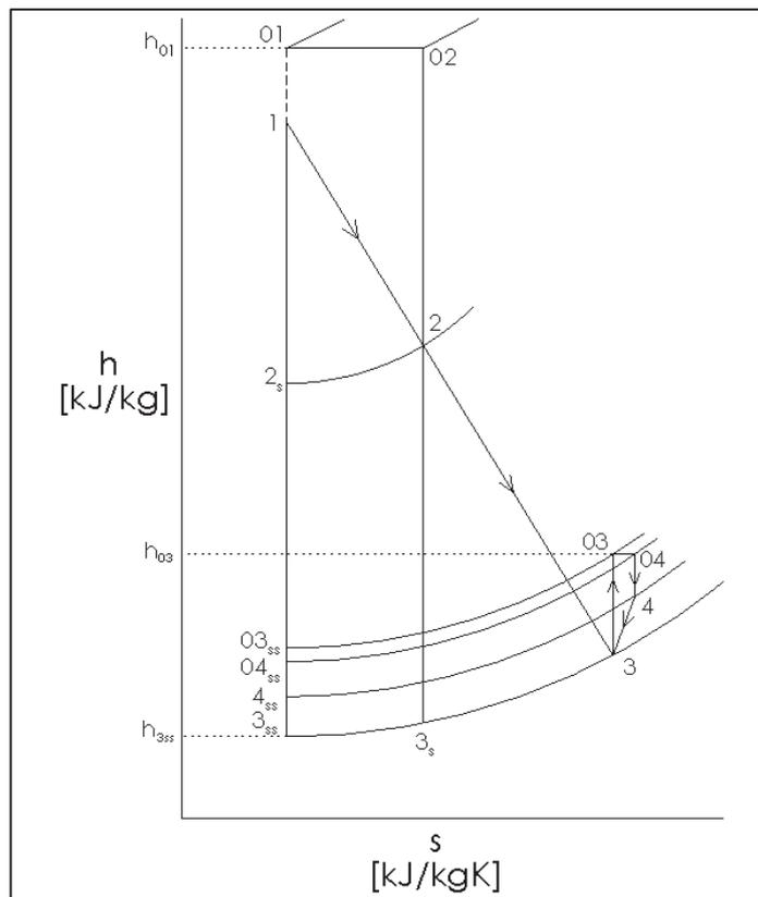
Figure 3 - Mollier diagram (adapted from [15]).
