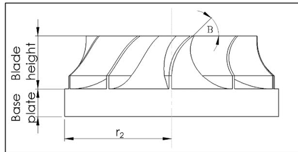
Figure 5 -Blade profiles of turbine rotors.
