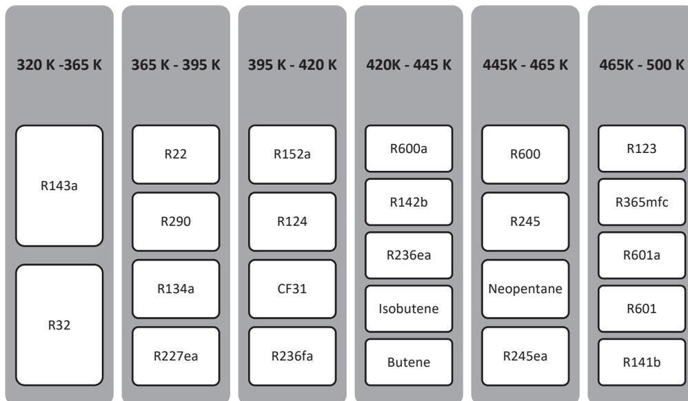
Figure 1 - Organic fluids at various temperatures for application in ORCs (adapted from [12]).
