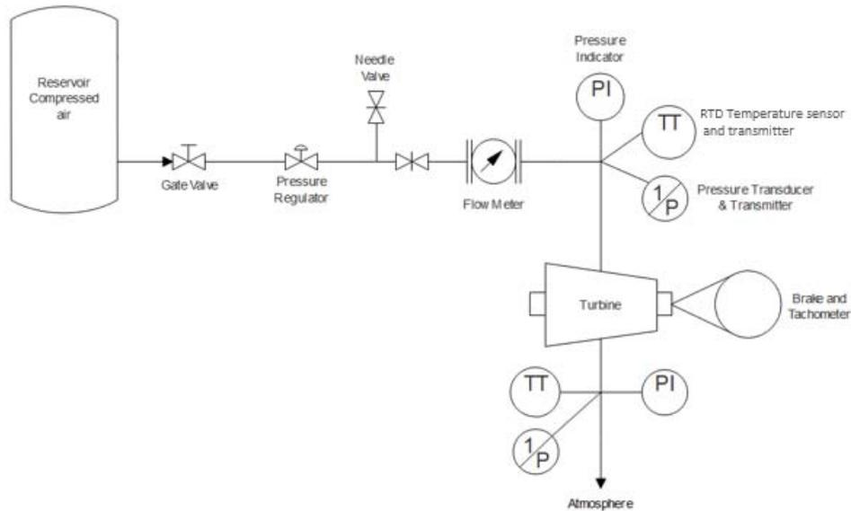
Figure 7 - Process flow diagram of the experimental setup.
