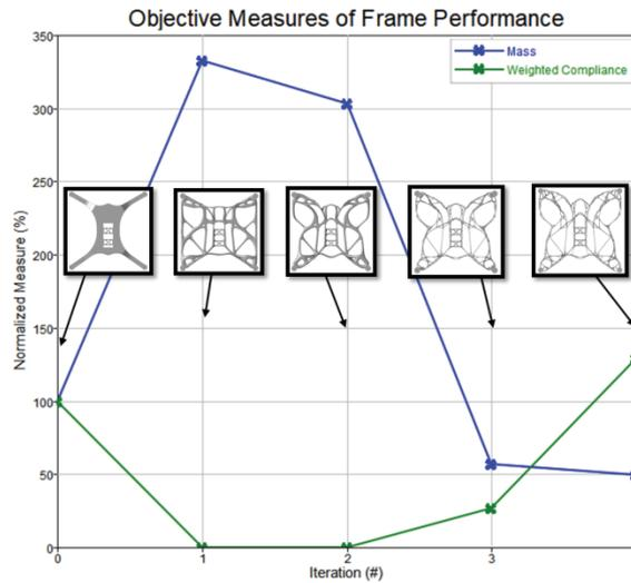
Figure 7: The normalized mass and stiffness trends through the design process.
