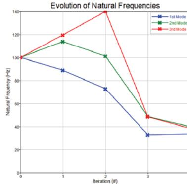
Figure 2: Evolution of the first three UAV frame natural frequencies.
