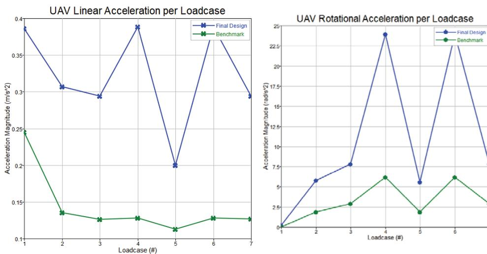
Figure 1: UAV accelerations per load-case for selected design iterations.
