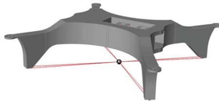
Figure 3: A concentrated mass connected to the landing gear to ensure topology generation.
