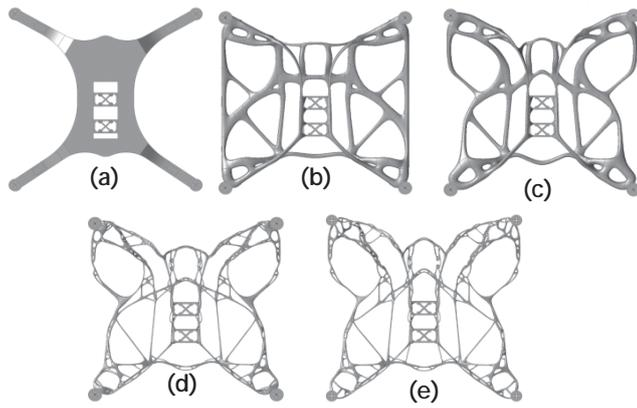
Figure 6: Selected design iterations that are used for evaluation. (a) Benchmark, (b)-(e) Iteration 1 to 4 respectively.
