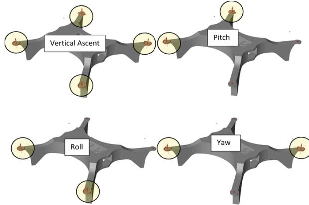
Figure 2: The load-cases for distinct UAV motions.
