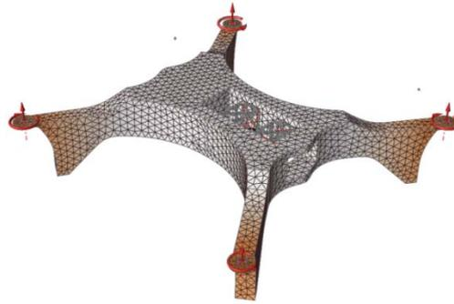
Figure 4: An illustration of the discretization of the UAV frame.
