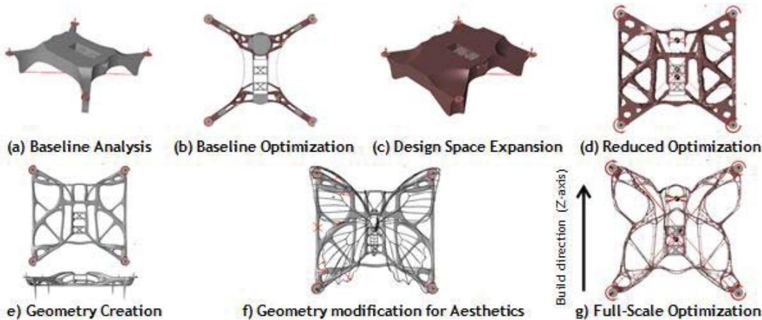
Figure 5: UAV frame design optimization Process.
