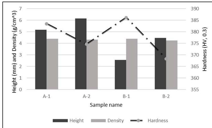
Figure 3: Microhardness variation, Density and Height measurements of the samples fabricated at different processing conditions.
