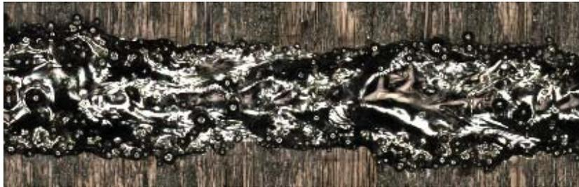
Fig. 2. Satellites at 170 W laser power and 0.4 m/s scanning speed.
