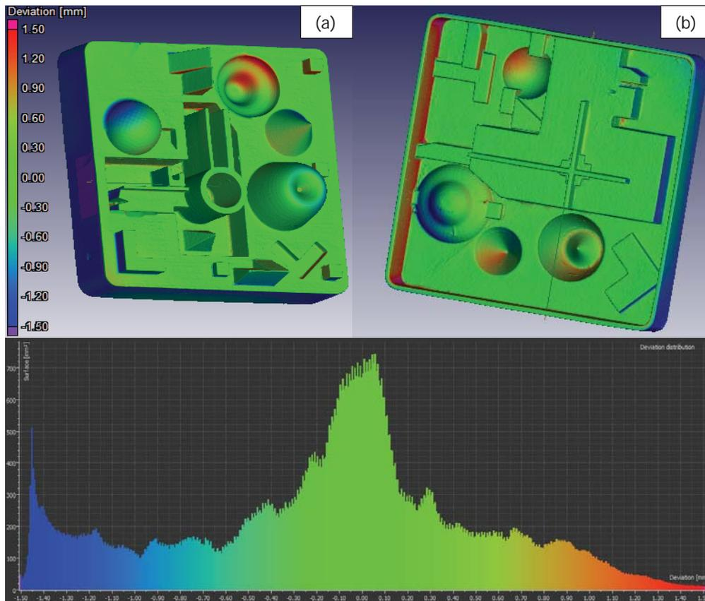
Figure 9: Casting results of the top (a), bottom (b) and the deviation distribution results from the PrimeCast® pattern (graph below (a) and (b)).
