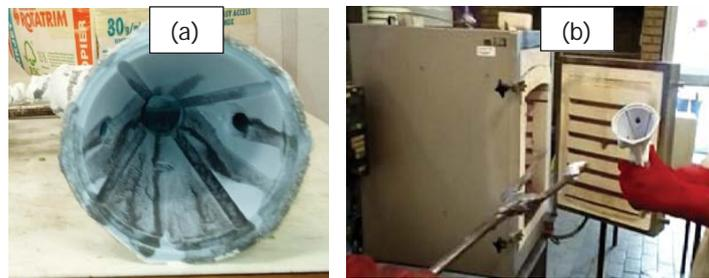
Figure 3: Shell with pattern residue (a) and White clean shell from the furnace (b).
