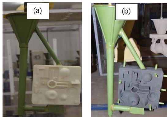
Figure 1: Sacrificial patterns with gating and vents: PMMA (a) and PrimeCast® (b).
