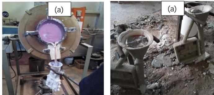
Figure 6: Pouring of the molten metal into the shell (a) and the shell with molten metal left to cool in air. (b)
