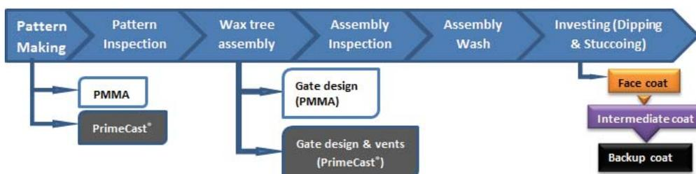
Figure 2: The flow diagram of mould making.
