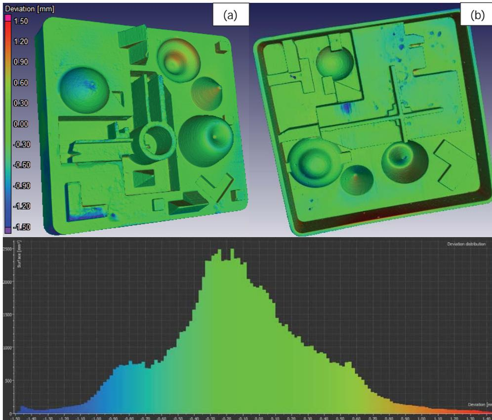
Figure 8: Casting results of the top (a), bottom (b) and the deviation distribution results from the PMMA pattern (graph below (a) and (b)).
