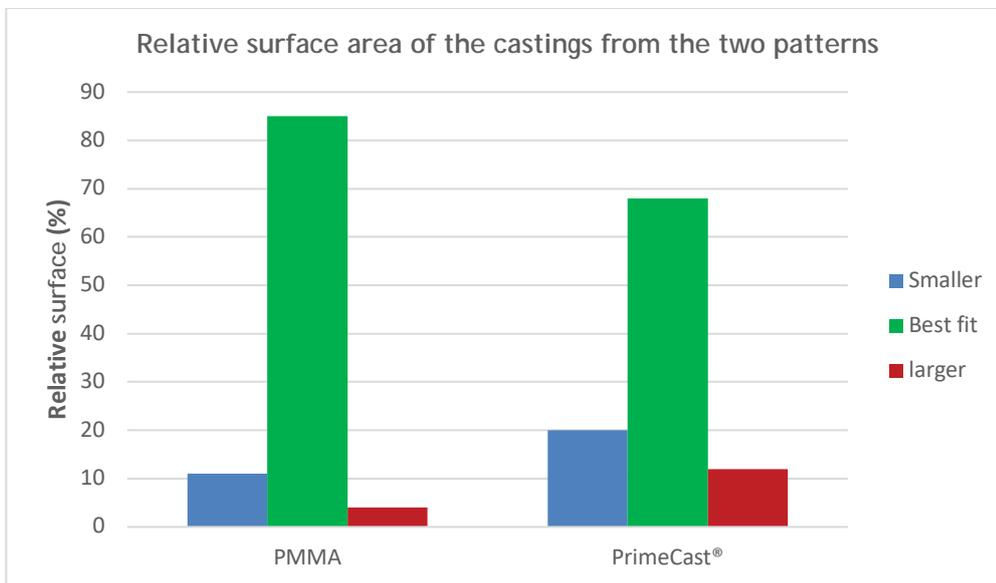
Figure 10: Comparison of relative surface area between the castings from the two patterns.
