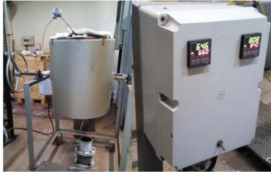
Figure 5: The furnace and the recorded temperature during melting of aluminium alloy.
