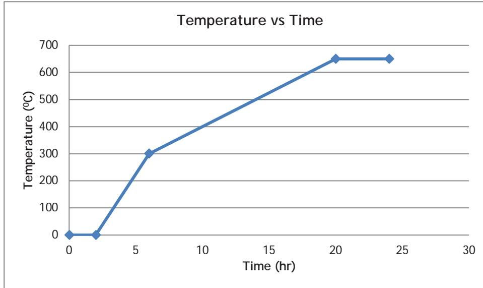
Figure 4: Temperature profile used for the burn-out furnace.
