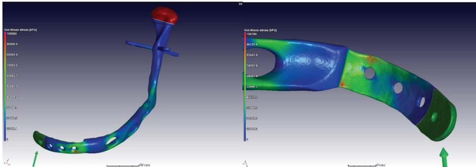
Figure 6: Mechanical simulation highlighting high stress areas in real part, using microCT data.
