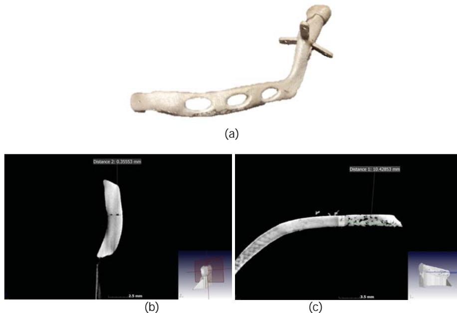
Fig. 5: Total view of Ti6Al4V mandible implant; CT scans cross-section of mandibular implant: parallel (b) and perpendicular (c) to the build direction.
