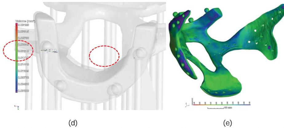
Fig. 4: Facial titanium implant step preview (a) CT scan of human skull defected area (b) implant attachment after the use of a cutting guide, and (c) full 3D assembly, showing placement of implant with lower jaw to ensure no implant error; CT scans reconstruction of the facial Ti6Al4V ELI implant: pores (d) and the deviation of the LPBF part from prescribed CAD sizes (e).
