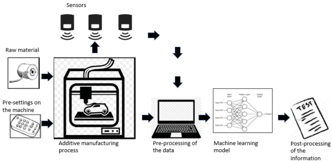
Figure 5. The process of developing machine learning models in additive manufacturing.
