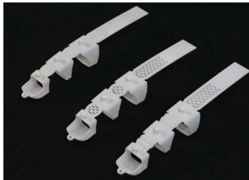
Figure 11: Solid, lattice and geometric wave structure live hinge printed concepts.
