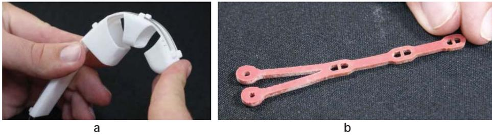
Figure 8: (a) Steel wire and guide and (b) rubber strip concepts to replicate tendons.
