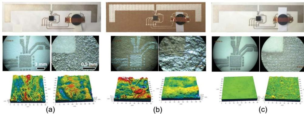
Figure 1: Assembled printed RFID sensing tags on low-cost substrates (110 mm x 30 mm) with corresponding microscope and LSM images (substrate = left, ink layer = right, scan area = 450 x 450  $\mu\text{m}$ ) for assessing printed features for a) standard printing paper, b) cardboard packaging and c) adhesive vinyl substrates.
