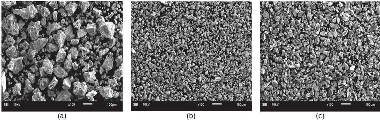
Figure 1: Particle morphology of starting powders: (a) 100 mesh TiHDH, (b) 325 mesh TiHDH, (c) 325 mesh 60Al40V master alloy.
