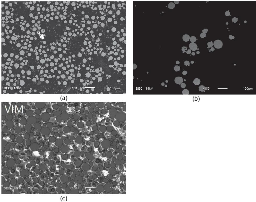
Figure 4: Polished sections of powders showing pores in some particles.
