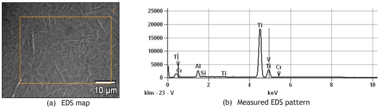
Figure 5: Microstructure and EDS analysis of powder particles.
