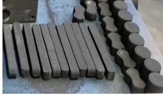
Figure 5: Transverse bars and tensile specimens.
