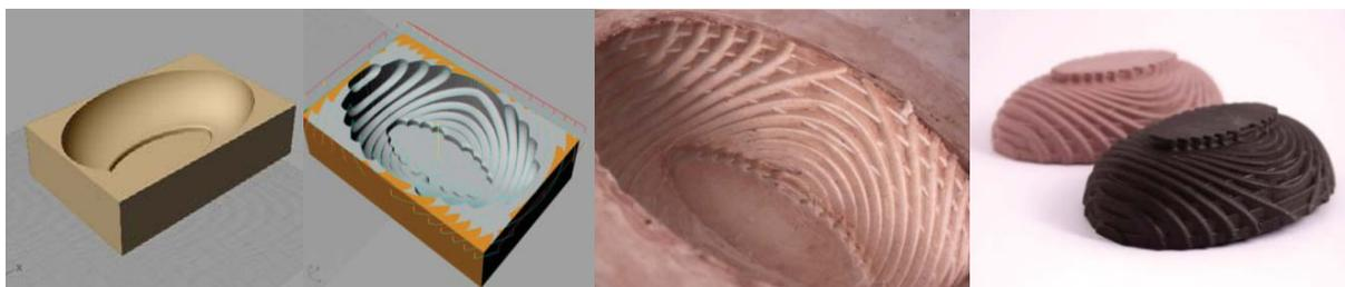
Figure 4: CAD file to final slip-cast and fired ceramic bowl. The Spiral CAM path and rough-cut levels are evident in the final product aesthetic.
