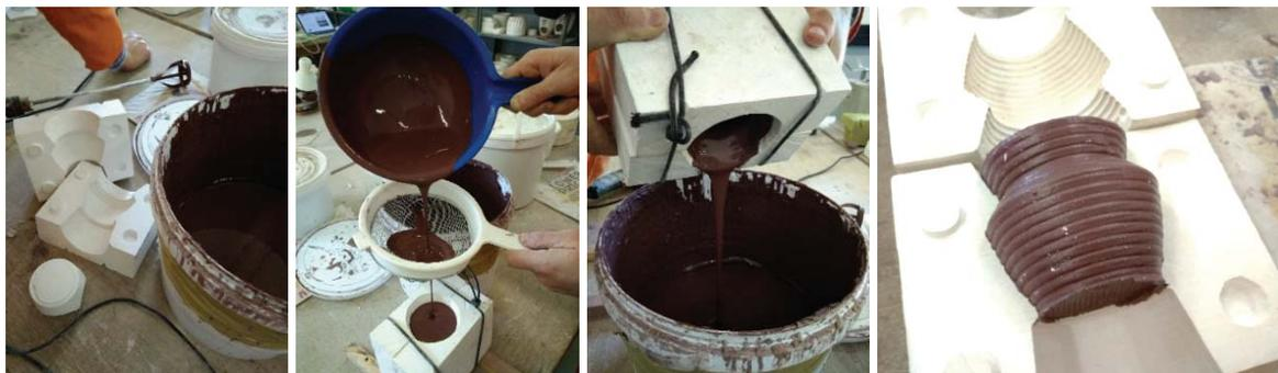
Figure 7: Slipcasting with black ceramic in the 3 part CNC mould.
