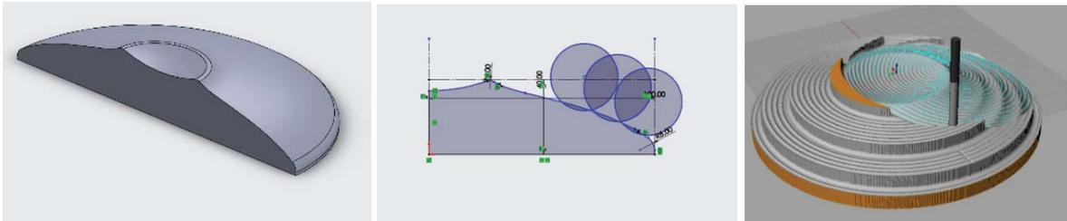
Figure 11: CAD modelling and CAM sequence prepared for the Dip-Casting form.
