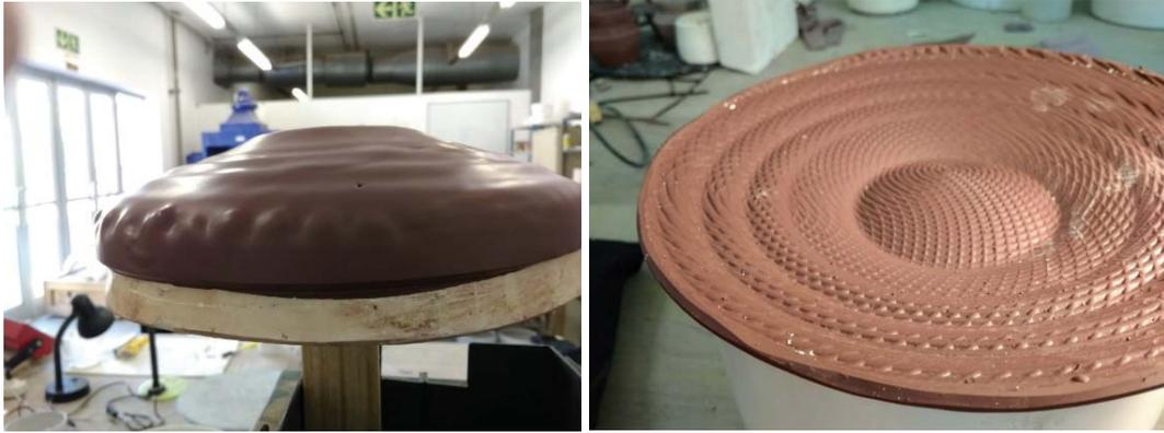
Figure 13: Dip cast for removed from positive mould showing surface texture created by cutting bit.
