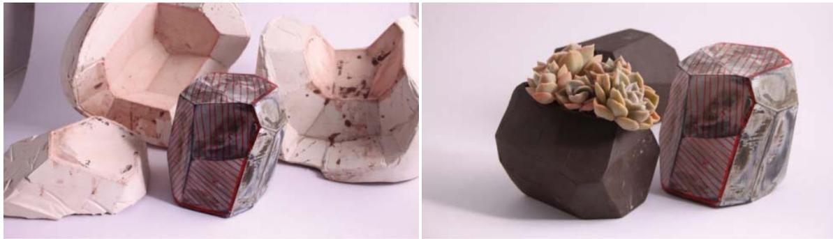
Figure 3: 3D printed pattern, 3 part slip-cast mould and hollow ceramic planter. Final planter cast in black slip and fired (right image).
