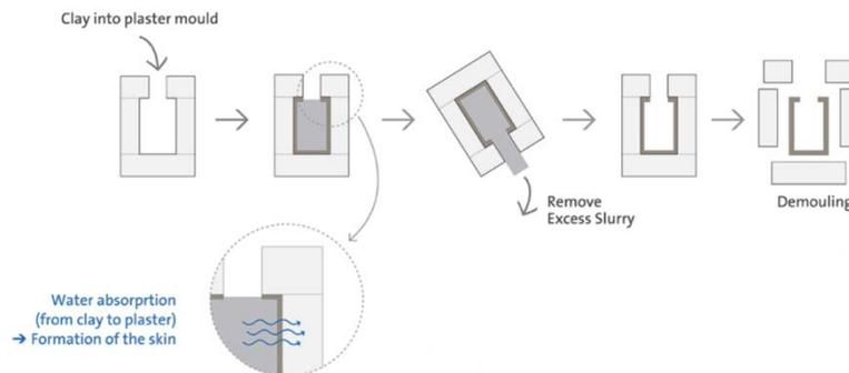
Figure 1: Slip Casting Process. [Online](#).
