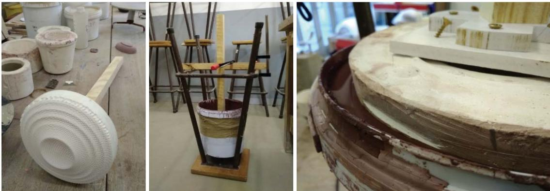
Figure 12: Dip casting the plaster form into the bucket of black slip. Barstool for added support.
