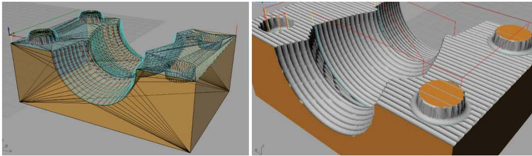
Figure 5: CAM cutting paths set to Rough cutting, and Parallel finishing (illustrated) Rhino and RhinoCam used for creating paths.
