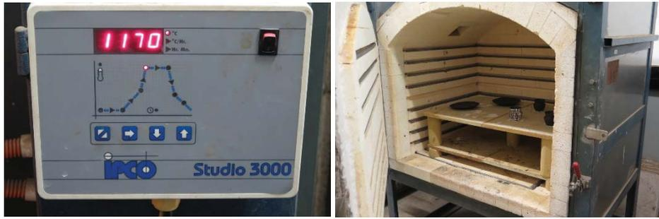
Figure 8: Firing the ceramic casts undertaken using ramp cycle totalling approximately 16 hours, with a maximum temperature of 1170°C.
