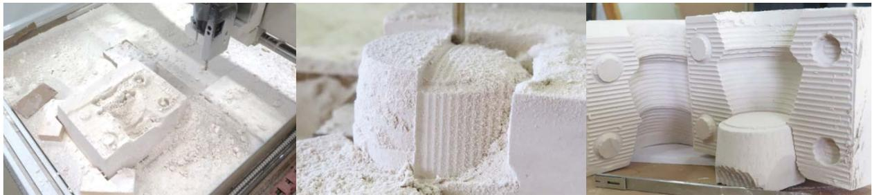
Figure 6: CNC cutting mould parts from Plaster of Paris blocks.
