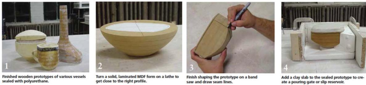
Figure 2: Mould Making Process, [Online](#).
