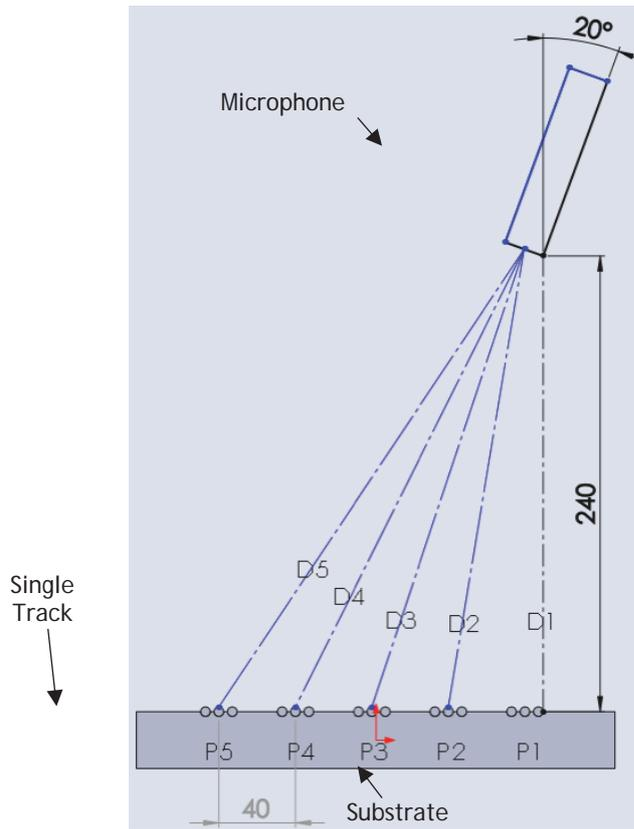
Fig. 2. Correctional view of system layout.
