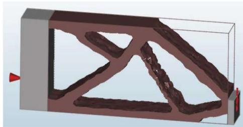
Figure 4: Facet geometry created from the TOP process[13],[14].
