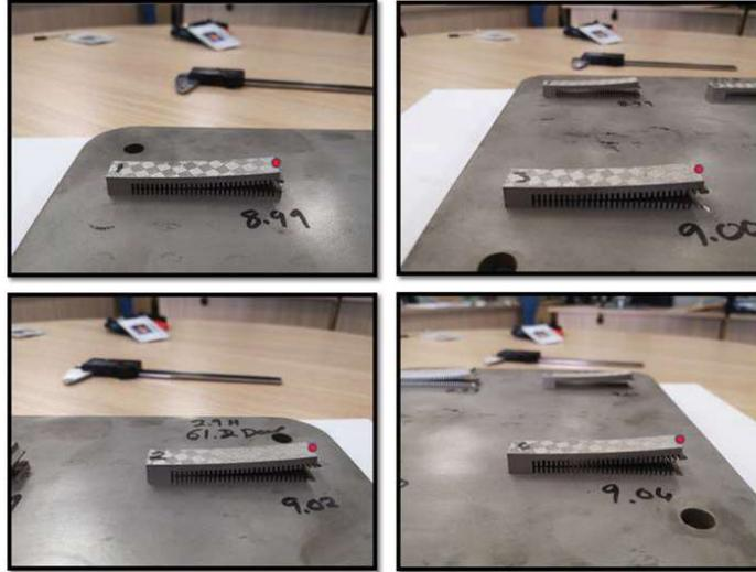
Figure 9: Cantilever samples after Cutting
