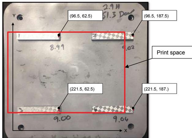
Figure 8: Distributed Samples across the build plate
