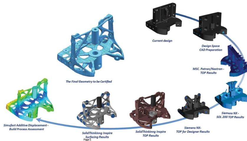
Figure 7: The results of the AM design cycle
