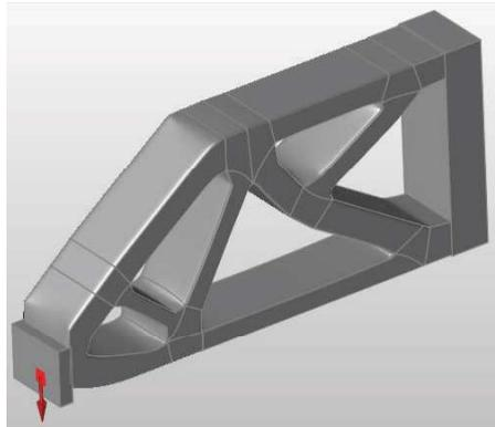
Figure 5: PolyNURB geometry[13],[14]
