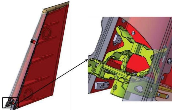
Figure 6: The Rudder assembly for the bottom bracket [17].
