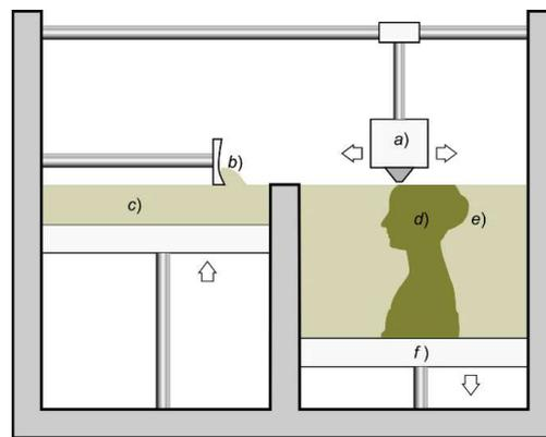
Figure 1 Powder bed Technology Components [10]
