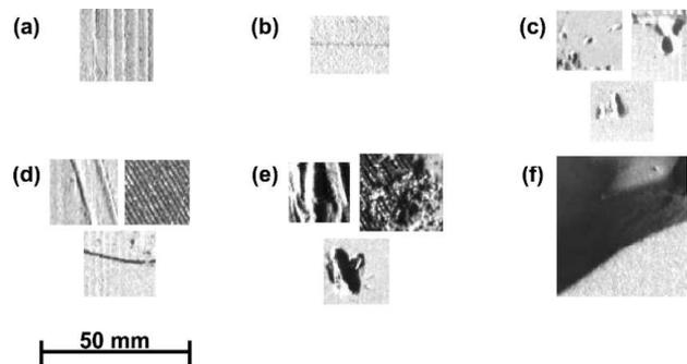
Figure 14 Powder bed defect types [14]
