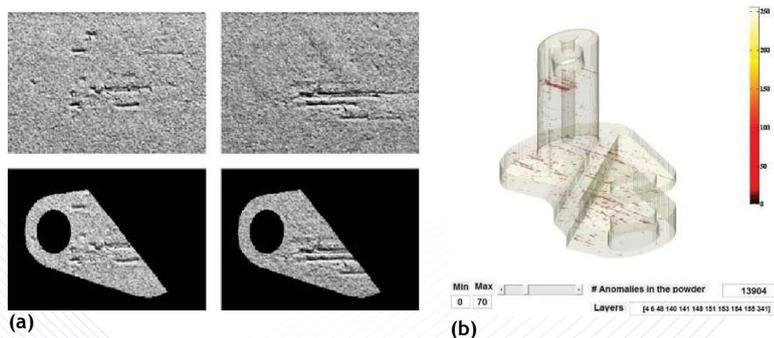
Figure 10 Re-coating errors and re-coating error 3D model [13]
