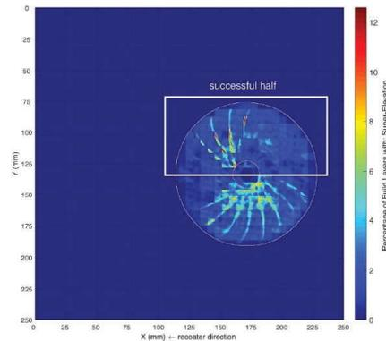
Figure 15 Heatmap of Super Elevation Defects [14]
