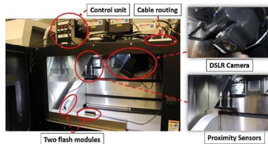
Figure 8 Camera and Lighting setup [13]
