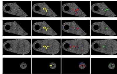
Figure 11 Detected Part Fusion Defects [13]
