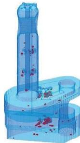
Figure 12 3D CT Model with defects indicated [13]
