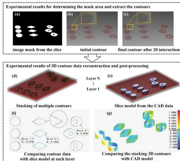
Figure 7 Comparison of Contour data to CAD model [12]
