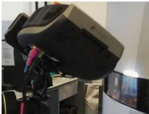
**Figure 3 Fringe projection scanner [11]**
