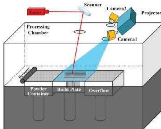
Figure 5 Camera setup for powder bed imaging [12]
