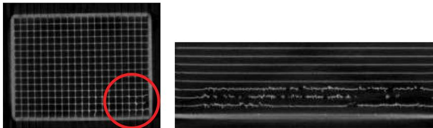
Figure 18: Scan 3, broken channels. Top and front view.
