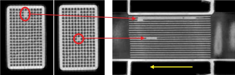
Figure 14: Scan 2, blocked channels. Top and front view.
