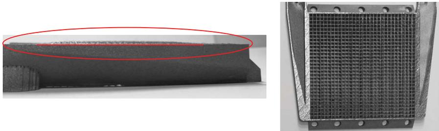
Figure 8: Design 3, 1<sup>st</sup> build attempt, side and top view
