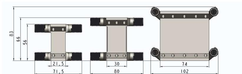
Figure 4: Size comparison of the three heat exchanger designs, front view
