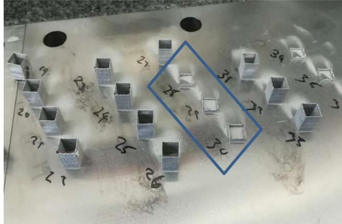
**Figure 2: Titanium tubes as built. The blue square shows the delaminated samples of poor quality**
