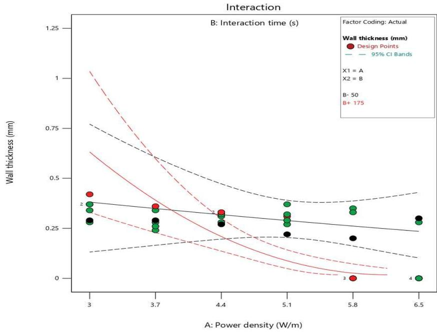
Figure 4: Response surface plot for wall thickness.
