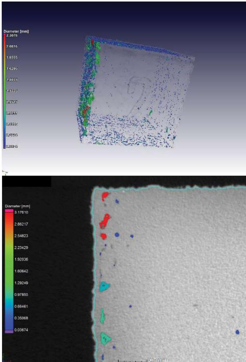
**Figure 7: Sliced Micro-CT images representative of the sample 2. The coloured markings show porosity concentrated near the surface**
