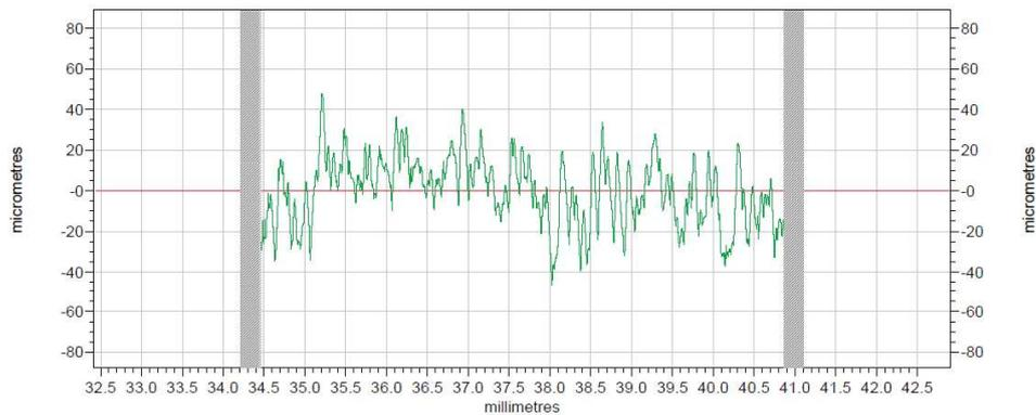
Figure 5: Surface finish profile of sample 25 showing an average line fitted for calculating the mean roughness (Ra)
