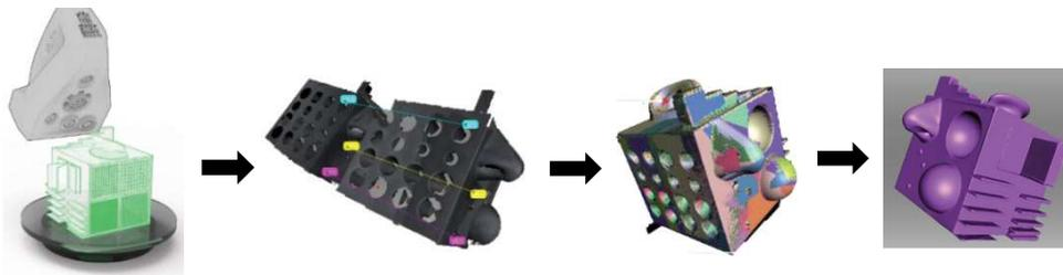
Figure 6: Hand-held scanning process of the test artefact.
