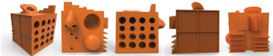
**Figure 8: Digital 3D model produced through Micro CT scanning of test 3D printed test artefact.**
