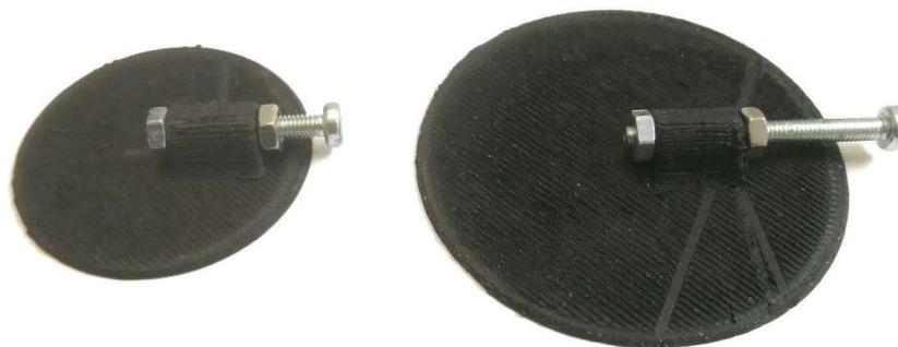
**Figure 2: The 3D printed electrodes with a stainless steel bolt to allow connection to the medical devices.**
