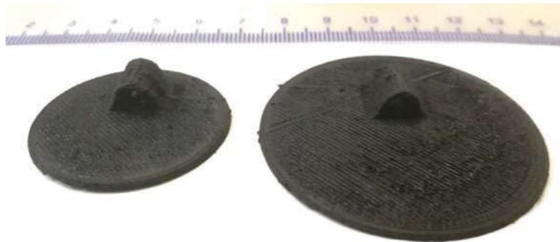
**Figure 1: The 35 mm electrode (left) and 50 mm electrode (right) that was 3D printed with conductive PLA.**
