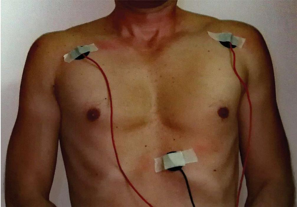
Figure 4: Position of the 3-electrode configuration on a person's chest
