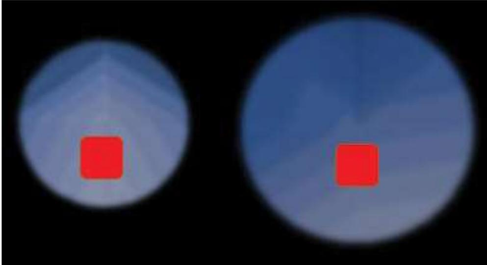
Figure 5: 35 mm electrode (left), ranging from 592 Ohms (lightest) to 862 Ohm (darkest). 50 mm electrode (right), ranging from 522  $\Omega$  (lightest) to 992  $\Omega$  (darkest). Red point indicates electrode lead connectivity point from which measurements were made.
