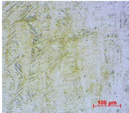
**Figure 5: Microstructure of SLM Ti6Al4V [8].**
