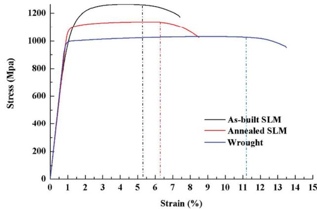
Figure 2: Stress-strain curves of As-built SLM Ti6Al4V, Annealed SLM Ti6Al4V and wrought Ti6Al4V [28].
