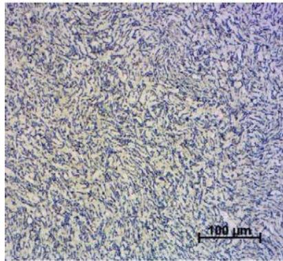
Figure 4: Microstructure of wrought Ti6Al4V [8]
