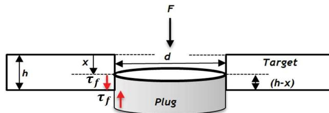
Figure 1: Plugging under ballistic impact
