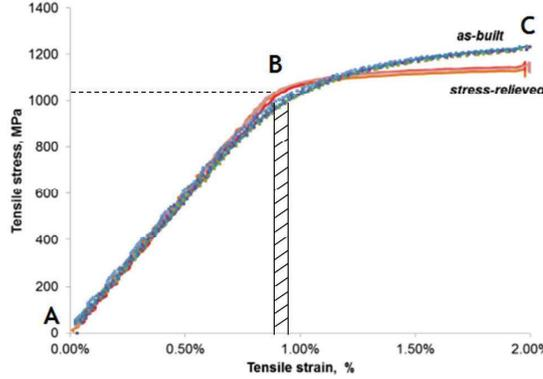
Figure 3: Stress-strain diagram of DMLS Ti6Al4V (ELI) [26].
