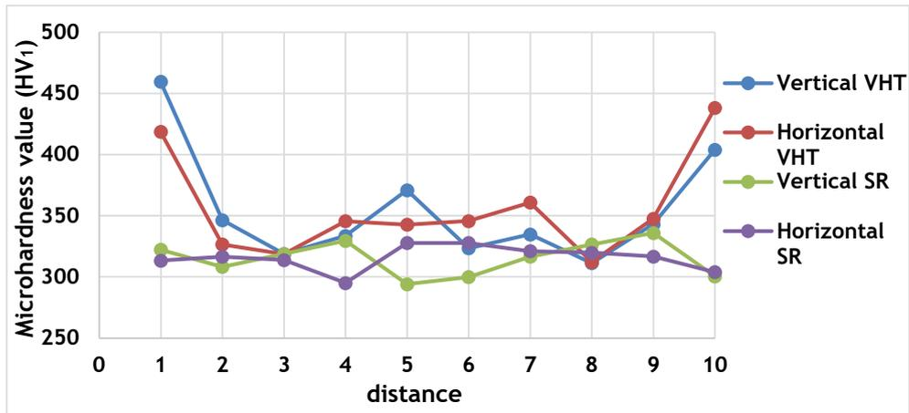
Figure 4. Hardness profile of VHT (horizontal-vertical) and SR (horizontal and vertical) porous Ti6Al4V structures.
