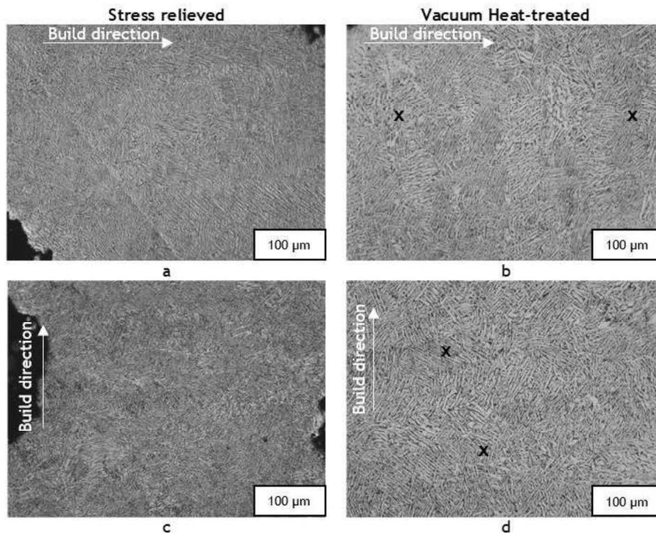
Figure 2. Optical micrographs of Horizontally built-in stress relieved condition (a), vacuum heat-treated condition (b), Vertically built-in stress relieved condition (c) and vacuum heat-treated condition
