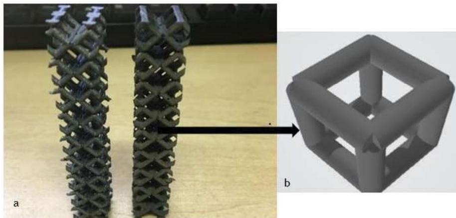
Figure 1. Front view of the Ti6Al4V porous structure a) and the CAD model of the porous structure b).
