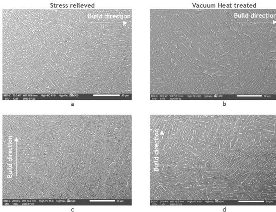
**Figure 3. SEM micrographs of Horizontally built-in stress relieved condition (a), vacuum heat-treated condition (b), Vertically built-in stress relieved condition (c) and vacuum heat-treated condition.**
