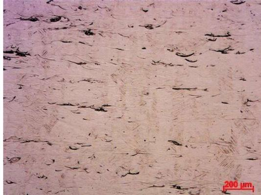
**Figure 1:** Etched by Kroll's reagent cross-section of *in-situ* alloyed L-PBF Ti6Al4V ELI-1.38wt.%Cu sample. Dark colour shows Cu-rich areas (confirmed by SEM-EDS analysis). Data from [4].
