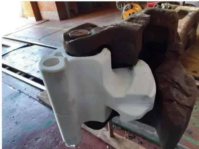
Figure 7: Knuckle prototype fitment trial
