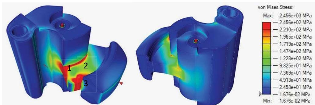
Figure 3: Generic design von Mises stress analysis
