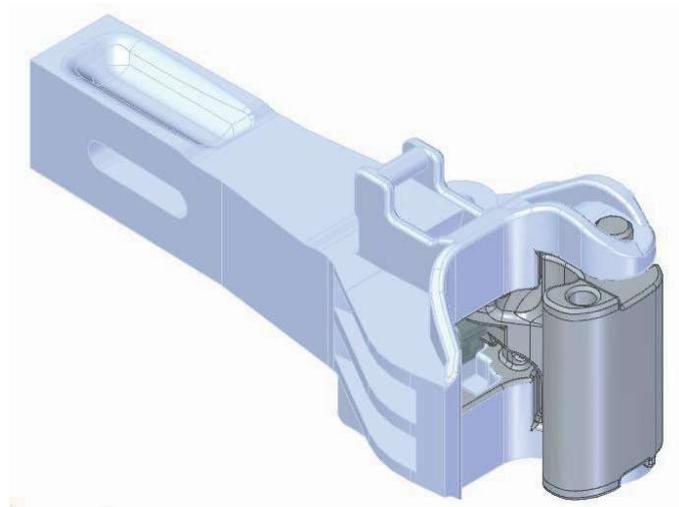
**Figure 1: Knuckle (grey) and coupler assembly**
