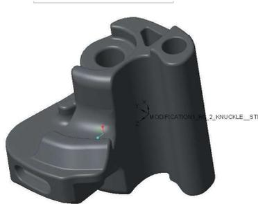
Figure 6: New design of the knuckle
