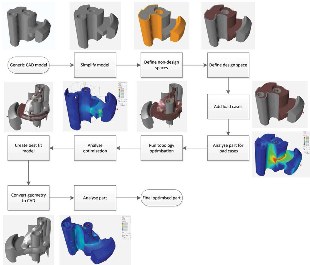
Figure 2: Process flow for the topology optimisation of the knuckle
