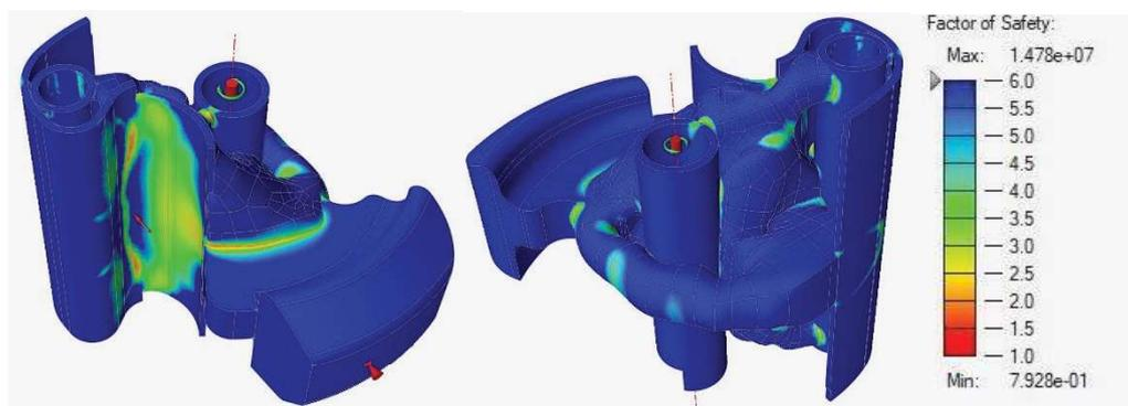
**Figure 5: FoS for optimised part in Grade E steel**
