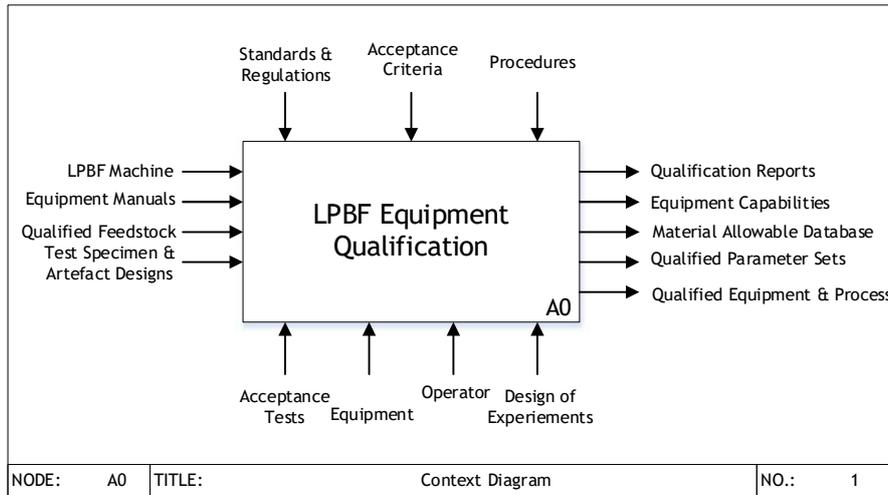
Figure 2: LPBF equipment qualification context diagram (A0 parent diagram).
