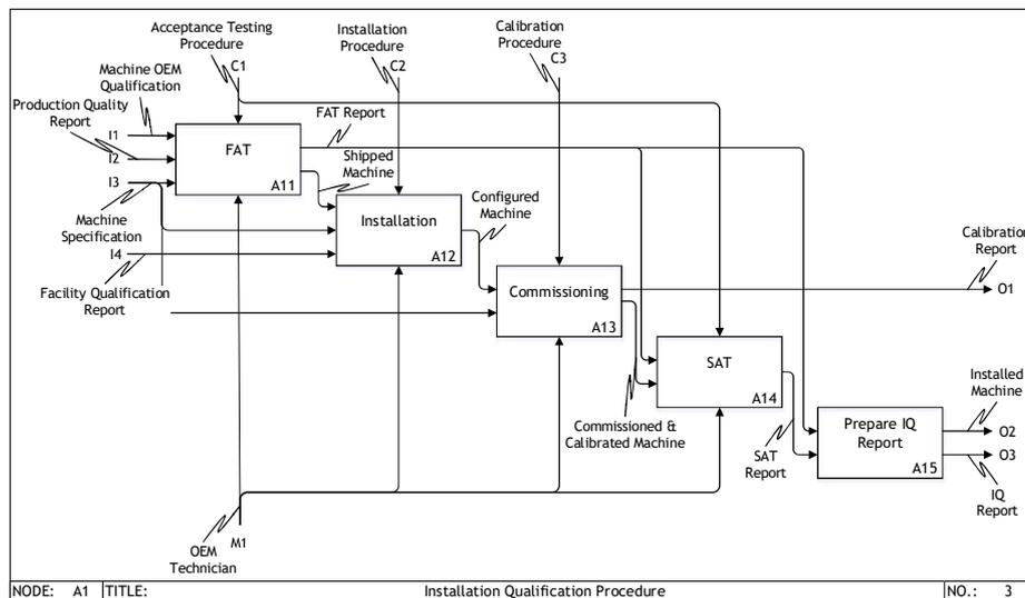
Figure 4: Installation Qualification procedure.
