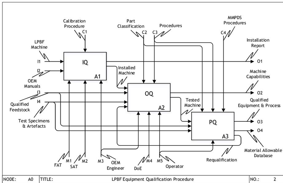
Figure 3: High-level LPBF equipment qualification procedure (A0 child diagram).
